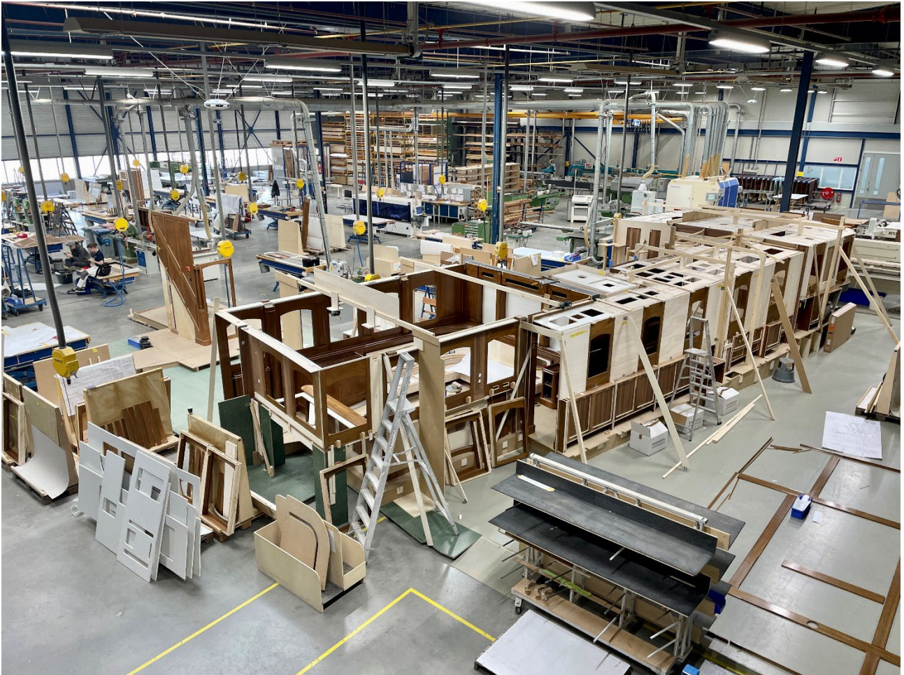
THE NEW MAIN DECKHOUSE AND BRIDGE DECKHOUSE INTERIOR UNDER CONSTRUCTION
