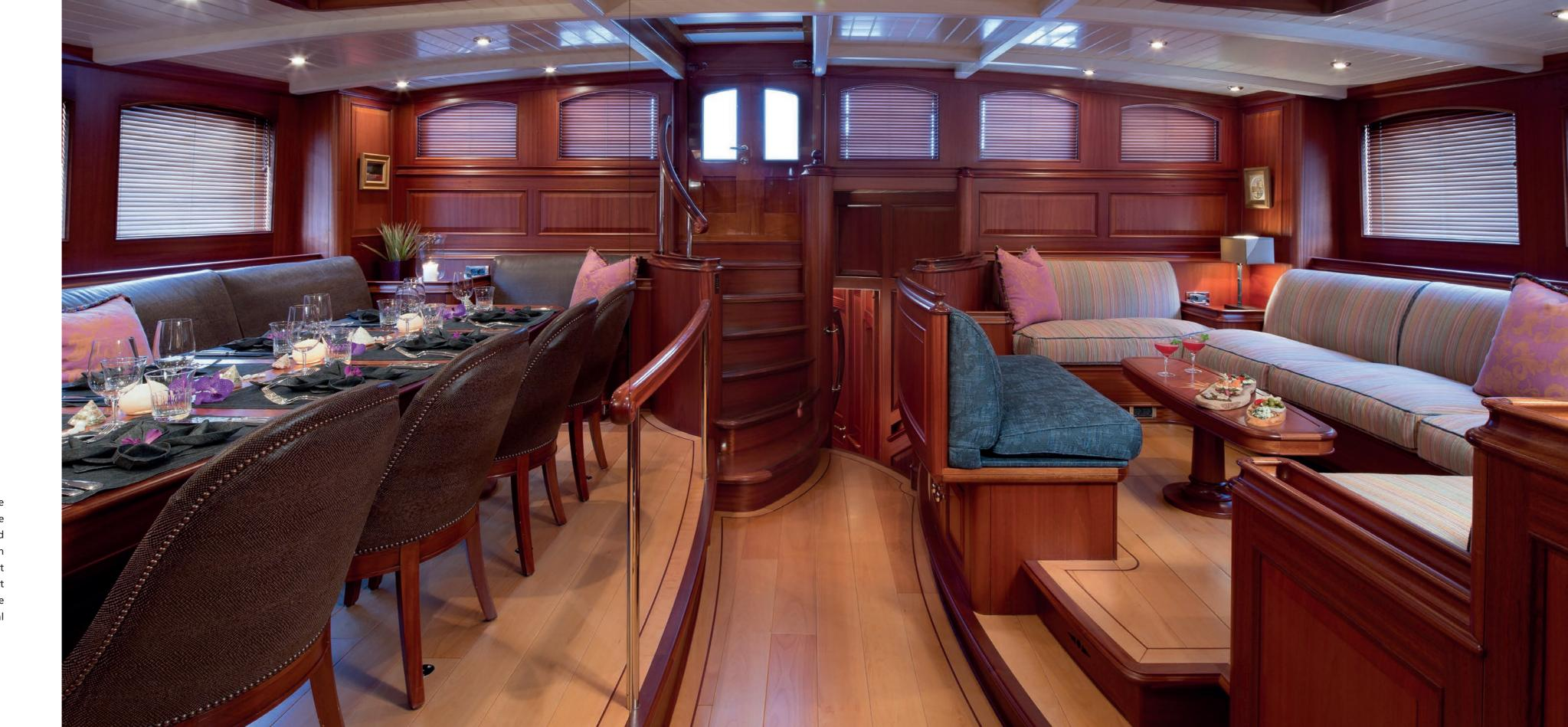
The main deckhouse floor has been raised to one level and provides an enhanced outlook. The entire interior, including the nav station, was taken out and a new design installed. The deckhouse looks much larger, the traffic flow is better and the natural light has improved. A new classic looking bar has been built on the portside and a couch occupies the space of the nav station, while smaller dining tables and casual seating maximize flexibility.
